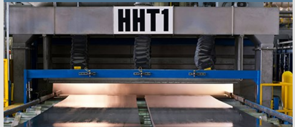
Horizontal Heat Treat (HHT) furnace at our Trentwood rolling facility.
